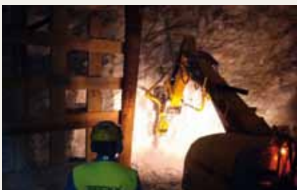
Breaking out talc in Italy. Brokk 260 with breaker SB302 and wide chisel.
