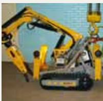
Brokk 90 with lifting frame and steel shears in Ukraine.
