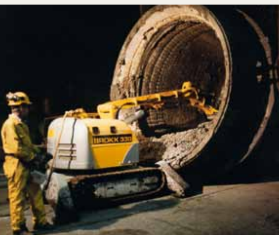
Ladle cleaning. Brokk 330 with SB 452.
