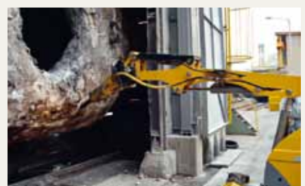
Cleaning torpedo opening. Brokk 180 with SB 202 in Posco, South Korea.
