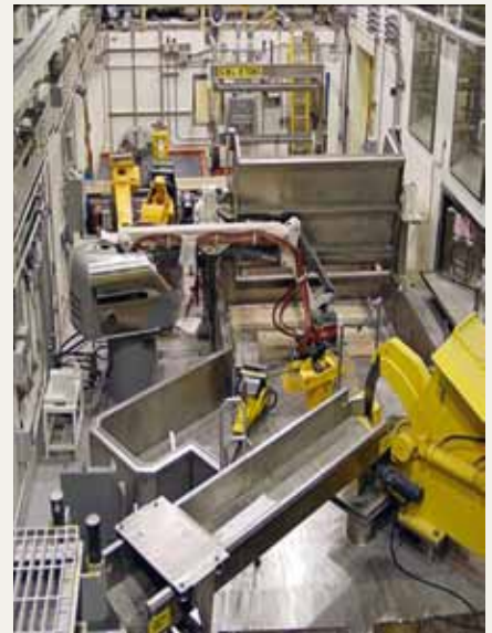
Sorting radioactive waste. Stationary Brokk 330 with sorting grapple.
