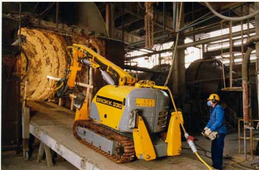
Entering a Bricking Solutions aluminium ramp. Brokk 330 with SB 300.
