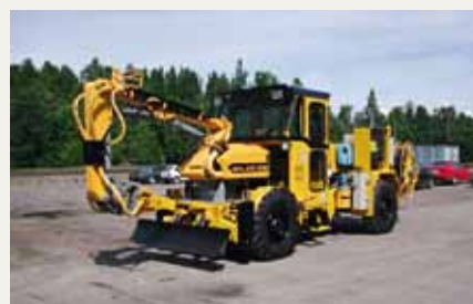
Brokk 330M for scaling mounted on a GIA carrier.
