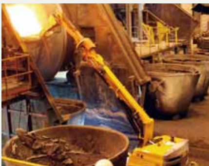
Copper converter mouth cleaning with Brokk 800 and a special designed heatprotected breaker in Sweden.
