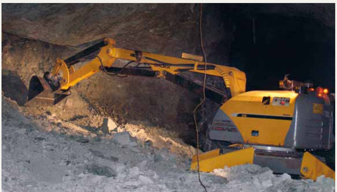
Underground digging in a narrow-vein gold mine in Australia. Brokk 330 with bucket.
