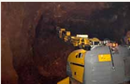
Breaking out bauxite. Brokk 330 with hammer SB 452 in Greece.
