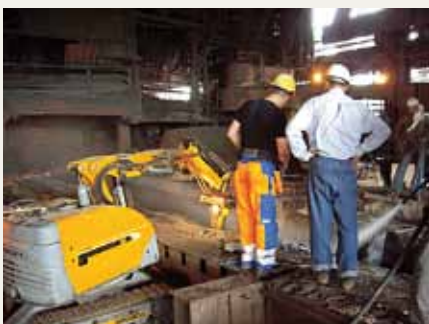
Blast furnace runner cleaning. Perfect view for the operator!
