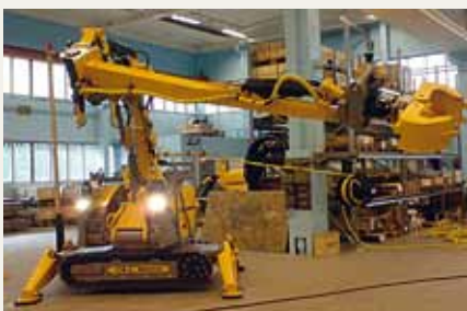
Picking and reducing waste from vaults. Brokk 400 with extra arm and sorting grapple in China.
