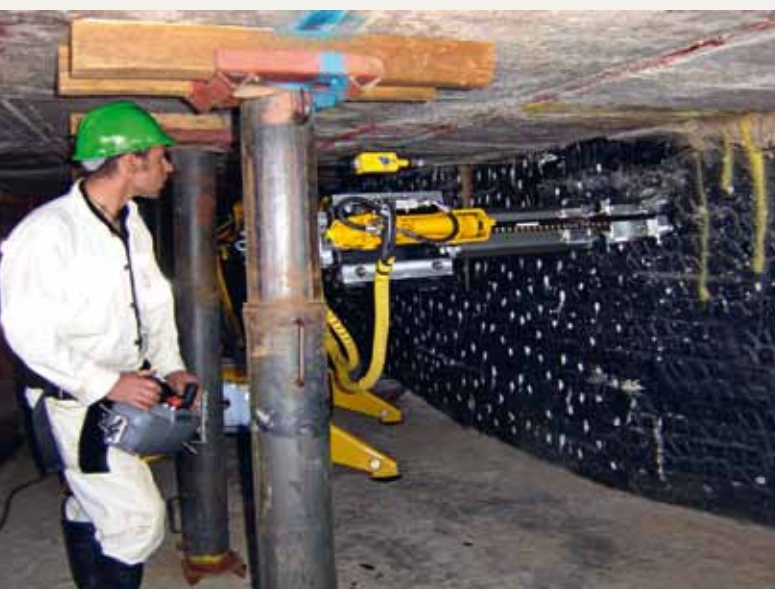
Face drilling in a narrow space. Brokk 90 with BSD-80 hydraulic drill in South Africa.
