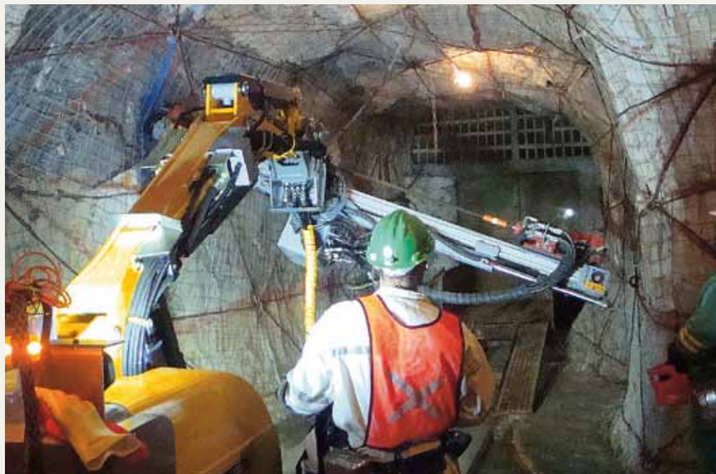
Blast hole drilling and anchoring. Brokk 180 with MMB260 hydraulic rock drill.
