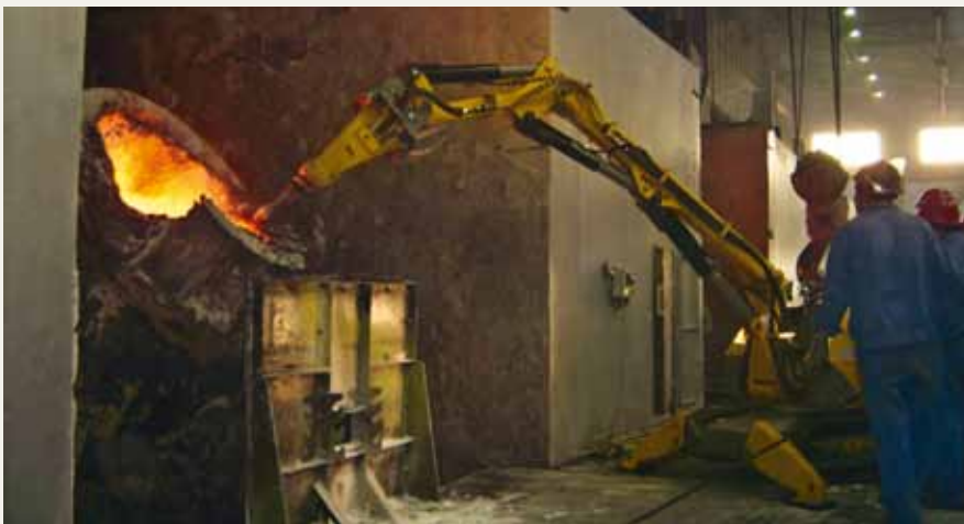
AOD furnace mouth cleaning. Brokk 330 with SB 300 in Taigang, China.
