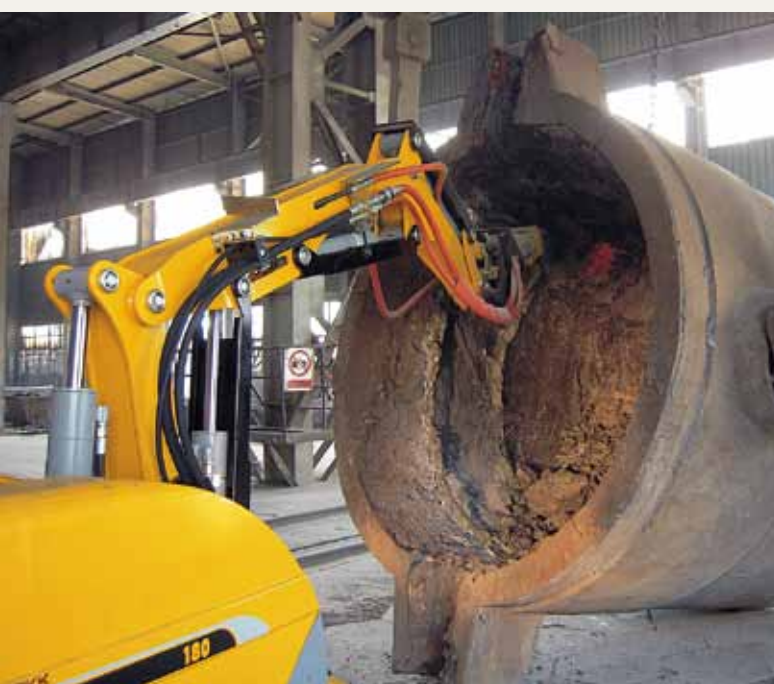
Ladle cleaning. Brokk 180 with SB 202 in Ferroalloy plant.
